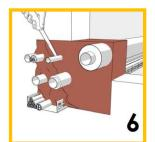
**5.** Fill the opening from back to front. In this process build up the foam from bottom to top, always guide the tip of the mixing nozzle above the foam so that the material does not stick or clog. After a work interruption longer than approximately 50 seconds the foam hardens in the mixing nozzle, which then must be replaced. Prior to changing the mixing nozzle, offload the dispensing gun, and carefully replace the mixing nozzle.
