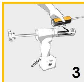
3.Insert the cartridge into the intended dispensing gun.
