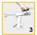
**3.** Insert the cartridge into the intended dispensing gun.
