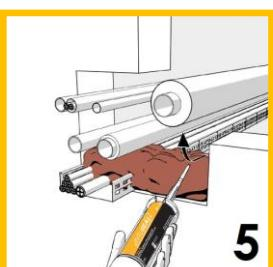
5.Fill the opening from back to front. In this process build up the foam from bottom to top, always guide the tip of the mixing nozzle above the foam so that the material does not stick or clog. After a work interruption longer than approximately 50 seconds the foam hardens in the mixing nozzle, which then must be replaced. Prior to changing the mixing nozzle, offload the dispensing gun, and carefully replace the mixing nozzle.
